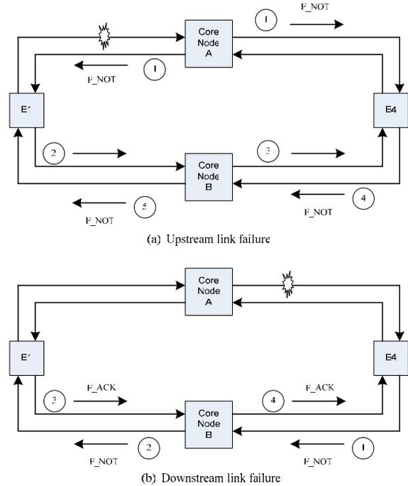
Figure 3 Signaling control process
